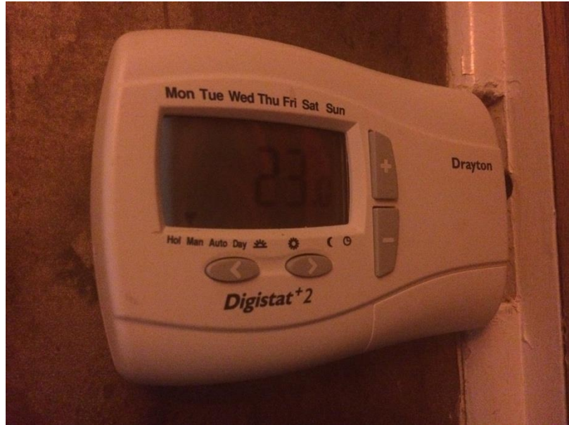
Figure 4 Photograph of a Drayton Digistat+2 / +2RF Programmable Room Thermostat.
